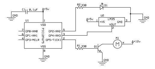
Notes: The Temperature sensor U2 needs to be located next to the item being monitored. As the temperature increases the motor duty cycle will increase.
